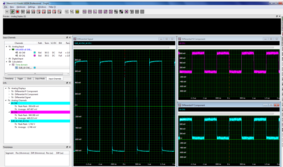
Figure 2: Using the subtraction function to combine two differential components into a differential signal.
