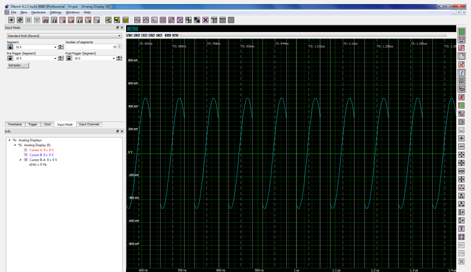
Figure 6: A test of the digitizer's re-arm time in multiple acquisition mode showing the capture of every cycle of a sine wave with an 88 ns period.
